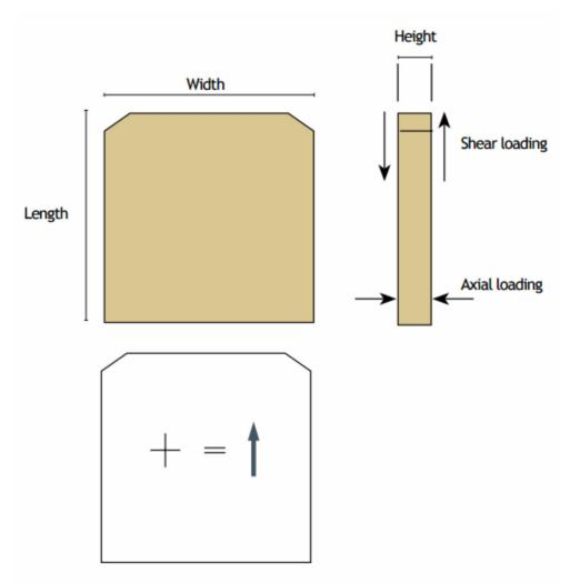
A positive voltage on one electrode leads to a relative displacement of this electrode towards the chamfered edge. This displacement is recorded as positive.
