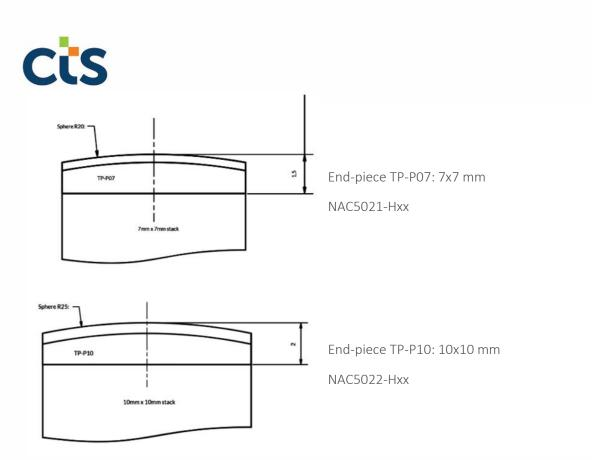
The design is compact, with spherical caps providing some de-coupling, thereby releasing the requirements on alignment. The parts are low-magnetic and compatible with our other add-ons. End-pieces can be attached at one or both ends of a stack. They can be supplied with a short lead-time and are more cost-effective for small series.
