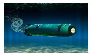
AUVs, otherwise known as underwater drones, are effective and economical alternatives for performing simple tasks without human supervision. Some AUVs perform the same tasks as ROVs, but with the advantage of covering a larger area. Common applications are surveys of the seafloor, mapping, pipe and structure inspection, recovery and research. For military and defense purposes, they can be used for activities such as mine countermeasures, anti-sub-marine warfare or payload delivery.
