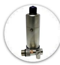
High Frequency Transducers offer frequency ranges from 30MHz to 150MHz. Applications include acoustic microscopy, flaw detection, and characterization of solder bumps in flip-chips in the microelectronics industry, high resolution thickness of meals down to 0.001" (0.0254mm), and high resolution surface wave imaging.
