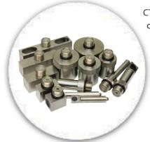
CTS' Immersion Transducers are specifically designed to operate in an immersion tank or with bubbler and/or squirter systems. They are manufactured with UHF waterproof connectors and can be designed with flat or focused lenses. All Immersion Transducers are offered in High Resolution (HR), General Purpose (GP), or High Performance (HP).
