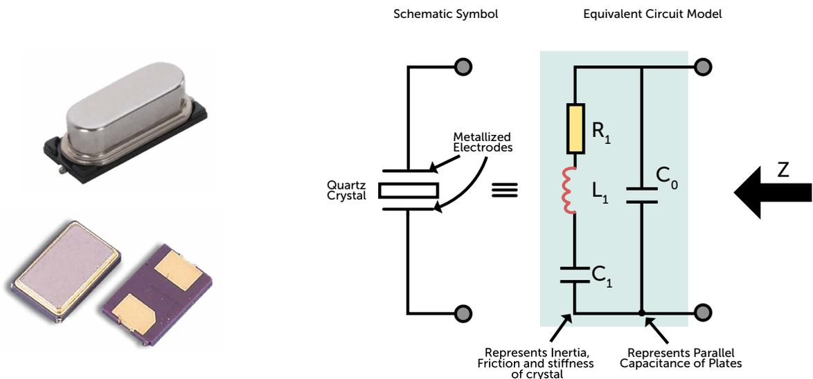
The equivalent circuit consists of the following parameters. All the parameters can be customized through design, but are tied together, so that a change to one parameter changes other parameters.
