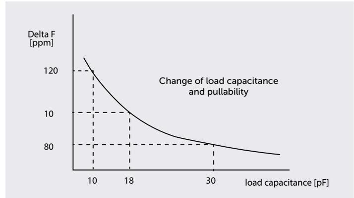
The Pullability of the crystal can be designed to meet customer's requirements. However, the pulling function varies with package size, electrode size, frequency, load capacitance range, and operating mode. Please contact CTS whenever you have a need for a pulling crystal.
