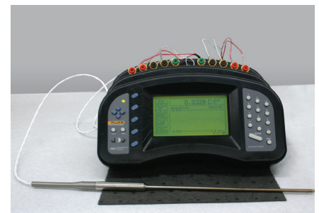
Figure 7. Thermometer readouts from entry-level systems to a primary standards model can achieve an accuracy of \pm 0.001^{\circ}\text{C} . Pictured above is a secondary platinum resistance thermometer (PRT), commonly used in calibration.
