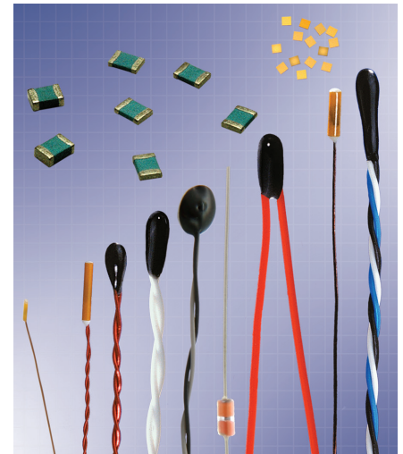
Figure 1. NTC thermistors are manufactured in a variety of sizes and configurations. The chips at the top of the photo can be used as surface mount devices or attached to different types of insulated or uninsulated wire leads. The thermistor element is usually coated with a phenolic or epoxy material that provides protection from environmental conditions. For applications requiring sensing tip dimensions with part-to-part uniformity and/or smaller size, the devices can be encapsulated in PVC cups or polyimide tubes.
