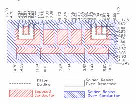
IMPORTANT: Please assure >=20mils (0.5mm) thickness of dielectric beneath the I/O Pads and the surrounding clearance zone down to the required ground plane.
