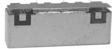
Part Dimensions: 25.7 × 5.3 × 6.7 mm • <2.6 g Materials: Ag plated ceramic block with tin plated brass shield
