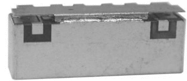
Part Dimensions: 25.9 × 5.0 × 6.7 mm • 2.2 g Materials: Ag plated ceramic block with tin plated brass shield
