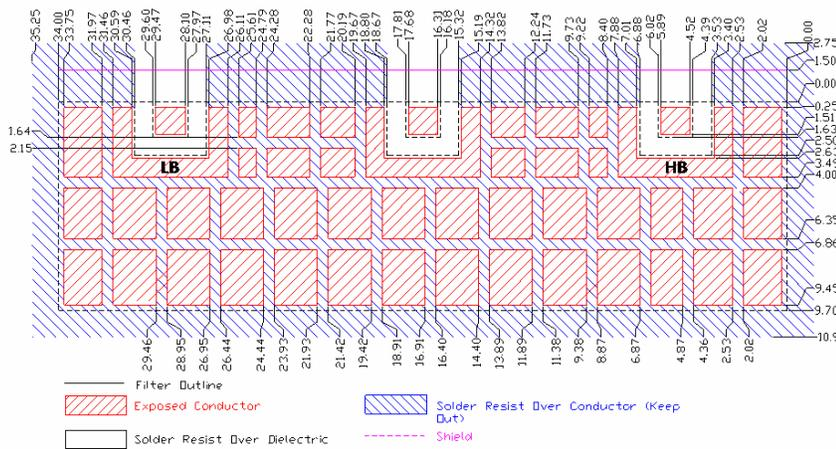
**IMPORTANT:** Please assure  $\geq 20$  mils (0.5mm) thickness of dielectric beneath the I/O Pads and the surrounding clearance zone down to the required ground plane.
