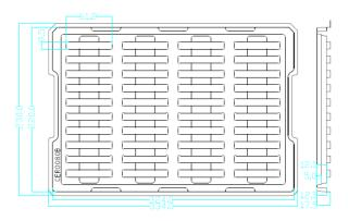
The trays have 40 slots each with one filter per slot. Boxes are packed with 4 Trays per box for a total of 160 filters per box.
