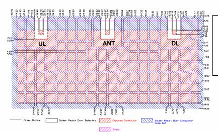
IMPORTANT: Please assure >=20mils (0.5mm) thickness of dielectric beneath the I/O Pads <u>and</u> the surrounding clearance zone down to the required ground plane.
