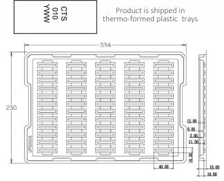
The trays have 60 slots each with one filter per slot. Boxes are packed with 9 Trays per box for a total of 540 filters per box.
