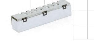
Part Dimensions:  $40.0 \times 10.5 \times 8.5$  mm • 10.7 g Materials: Ag plated ceramic block with tin plated brass shield
