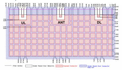
IMPORTANT: Please assure >=20mils (0.5mm) thickness of dielectric beneath the I/O Pads <u>and</u> the surrounding clearance zone down to the required ground plane.
