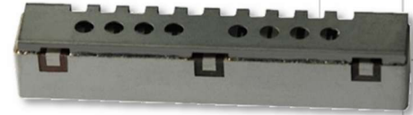
Part Dimensions: 44.2 × 5.2 × 8.5 mm • 5.2 g Materials: Ag plated ceramic block with tin plated brass shield
