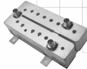
ESTIMATE Part Dimensions: 64 × 29 × 16 mm • <105 g (excl. connectors) Materials: Ag plated ceramic block with tin plated brass shield
