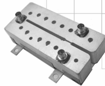
ESTIMATE Part Dimensions: 64 x 29 x 12 mm • <100 g (excl. connectors) Materials: Ag plated ceramic block with tin plated brass shield
