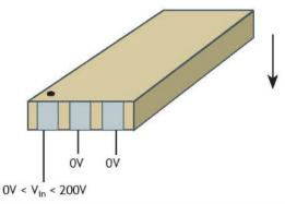
Note that it is similarly possible to control the bending in upwards direction by applying 0 V to the negative bias and a control voltage between 0 and 200 V to the positive bias and control electrode connected together.
