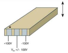
Note that if a different voltage reference is used, it is also possible to apply +200 V to the positive bias electrode, 0 V to the negative bias electrode and vary  $V_{in}$  between 0 and +200 V.
