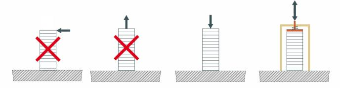
The mechanical load must be applied on the full surface of the actuator in order to avoid stress concentrations.
