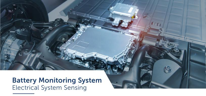
Battery Monitoring/Management Systems (BMS) monitor the physical variables of a battery, such as current, voltage and temperature and prevents the battery from operating outside its safe operation parameters. Monitored variables are used to check the battery state, to calculate secondary data, report that data, control its environment or for authentication.
