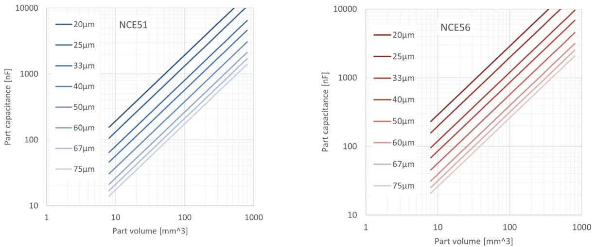
Fig. 7: Capacitance according to volume for standard layer thicknesses. NCE51 and NCE56 materials.
