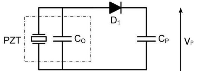
Fig. 4: Simple energy storage circuitry
