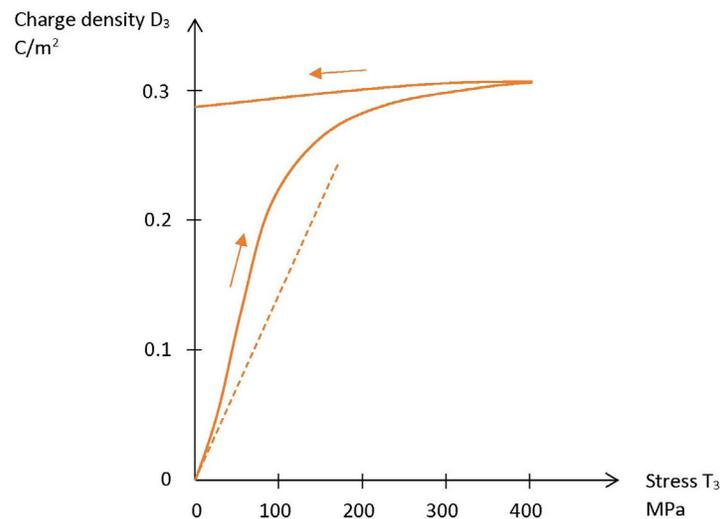
Fig. 1: Charge density versus stress, reproduced from [Zhou]. Solid line: published data. Dashed line: tangent at origin (linear piezoelectric equations).
