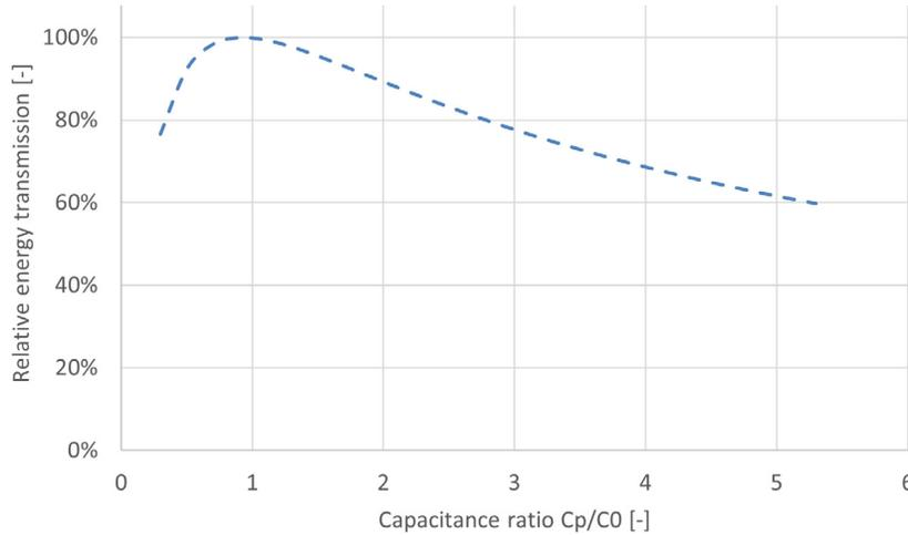
Fig. 5: Illustration of impedance matching, NCE51 material.
