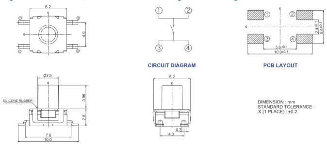
Figure 2 – 222MJV..., Surface Mount J Bend, Actuator Height 6.8mm
