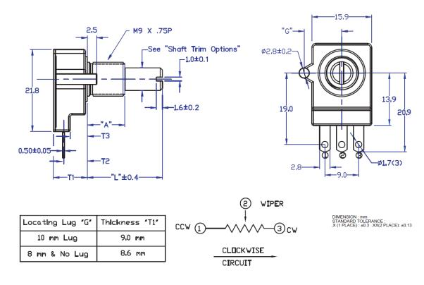
Series 282S Metal Shaft, Bushing Mount, Solder Lug "S" Type Terminal Formed to Rear
