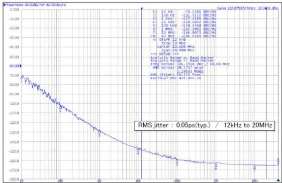
156.25MHz,  $V_{CC} = 3.3V$ ,  $V_{C} = 1.65V$ ,  $T_{A} = +25$ °C
