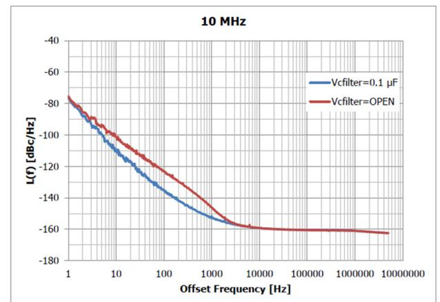
Figure 6 Vc filter Pin, Phase Noise Comparison
