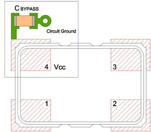
**Figure 1** Bypass Capacitor Connection
