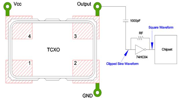
Figure 4 Waveform Conversion
