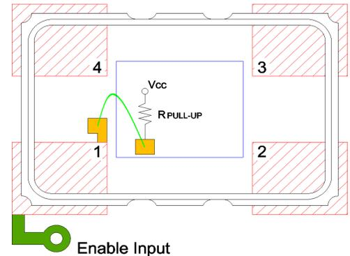
**Figure 2** Output Enable
