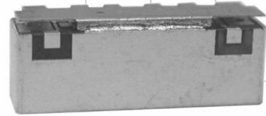
Part Dimensions: 25.9 × 5.5 × 6.7 mm • 2.8 g Materials: Ag plated ceramic block with tin plated brass shield
